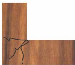
Crack arising due to L shape 90° cutting
